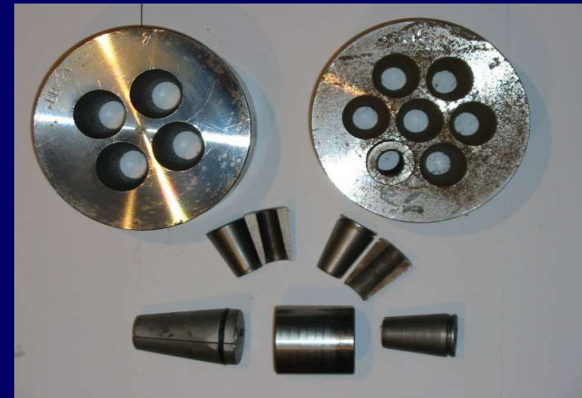
Anchor blocks and wedges
