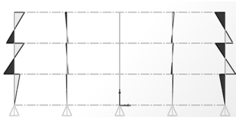
Column bending moment diagram due to full dead and live load on all spans
