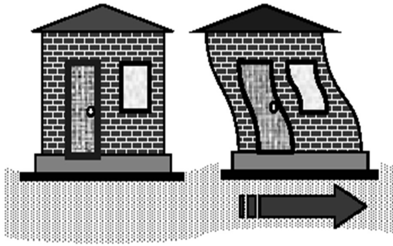
Figure 1: Effect of Inertia in a building when shaken at its base
