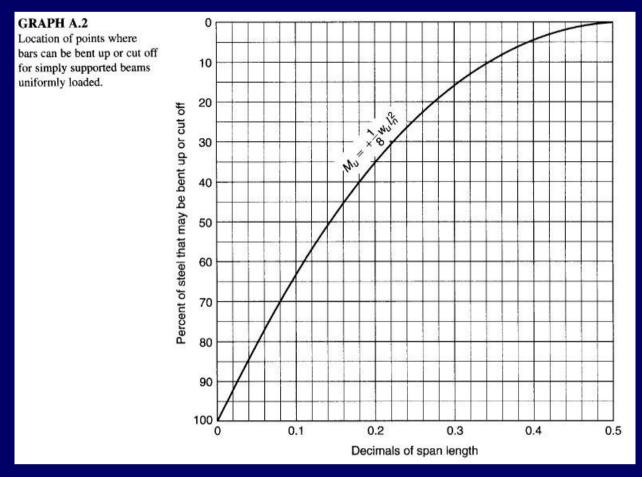
Exact curtailments lengths for simply supported positive moments (to be measured from face of the support)
