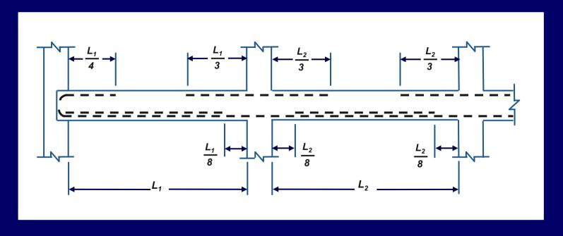
Cutoff for bars in approximately equal spans with uniformly distributed loads for 50% curtailment
